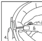
**WARNING: Excessive tightening may damage the clips.**
