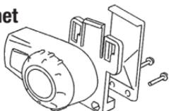
4. Tighten the screws to hold the clip firmly in place.
